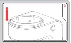
Turn the Feeder Chute (2) upside down and place into the Drive Sleeve (4).
