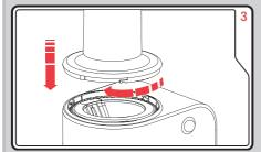
Place Feeder Chute (2) onto the Main Unit (6) so it falls into place and turn clockwise to lock in position.
