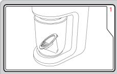
Place the Cutter Blade (3) inside each other and place inside the Beaker (8). Return the Beaker to it's position in the Base Unit (6).
