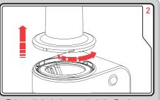
Twist anti clockwise to unlock the Feeder Chute (2), remove the Cutter Blade (3) (take care when removing the blade) remove Drive Sleeve (4) and wash in warm soapy water. Use a small brush to clean the blades if necessary.
