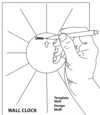
2. Ensure that there are no electrical wires or water pipes in the wall where you intend to screw/drill. Screw in an appropriate type of screw for the wall material. Hang the clock movement onto the screw.
