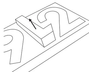
4. Place the first number (e.g. the number 1 of 12 o'clock) in the desired location and make a mark on the wall. In this example the tip of the minute hand is level with the top edge of the number. You may of course set the number in any other position to suit your needs.
