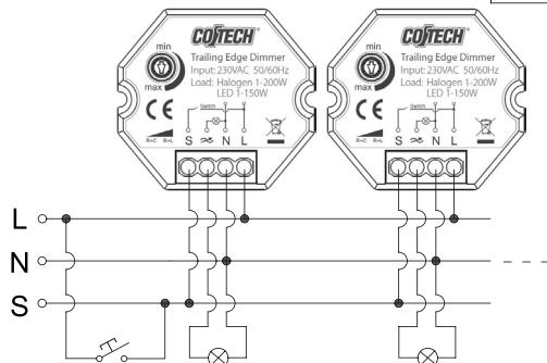
Thanks to their built-in synchronisation feature, multiple (up to 50) wall box dimmers can be controlled by the same spring-loaded on/off switch without the need for separate synchronisation between the wall box dimmers.
