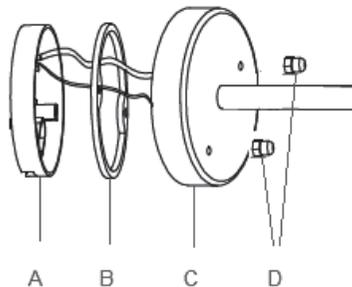
2. Loosen the two nuts (D) that hold the lamp base (C) against the wall mount (A).
