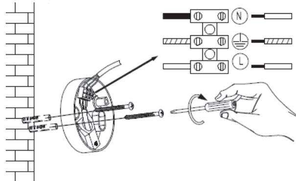
5. Pass the incoming feed cable through the rubber grommet in the wall mount.
