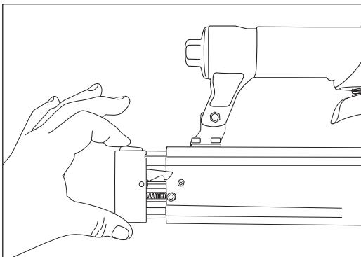
2. Place nails in the magazine, ensure that the tips point downward, and lie against the bottom of the magazine.
