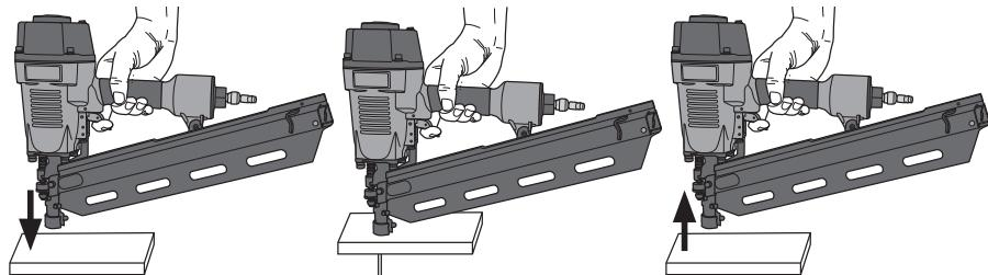
1. Hold tool firmly and press the trigger (3).
