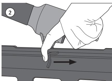
3. The magazine is open at the top. Load the nails. Before loading, check that the nails are clean and undamaged.
