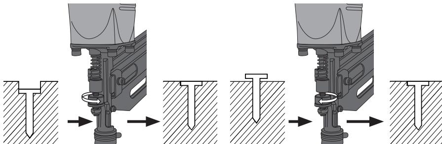
Turn the adjusting dial (2) clockwise to reduce the impact depth or counter-clockwise to increase the impact depth.
