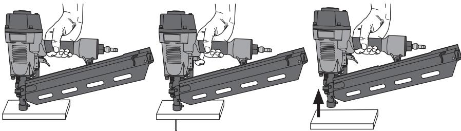
1. Hold the tool firmly (without holding down the trigger). Press the tool against the work surface.
