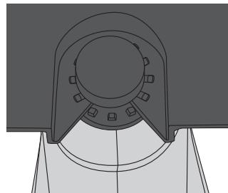
1. Flip the quick-release lever to its fully extended open position and pull the accessories bolt out enough to give the accessory clearance to slot into place.
