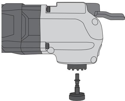
3. Press the accessory flush onto the retainer and flip the quick-release lever back to its locked and closed position.
