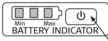
At full, 100 % charge, all three LEDs shine. At 90 % charge, one LED goes out and two LEDs will be lit. At 25 % charge, two LEDs are unlit and only one LED will be lit. If none of the LEDs are lit, the battery is completely discharged and needs charging.
