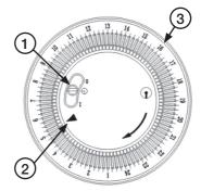
The convector heater is equipped with a 24-hour timer with pull-out segments for setting the on and off times. Each segment represents 15 minutes. The sliding timer mode switch can be set to 3 positions:
