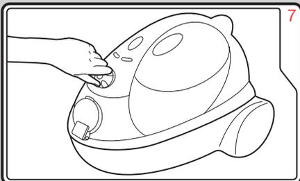
The variable steam control (5), varies the steam output. Turn the knob anti-clockwise as far as it will go for the maximum amount of steam, or clockwise to decrease steam output.
