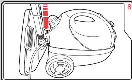
During use, the tubes and nozzle can be stored in the park position for short breaks whilst cleaning.
