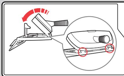
Remove the squeegee after use by holding the locking clip forward. Pivot the utility attachment up and unhook from the loops to lift it away.
