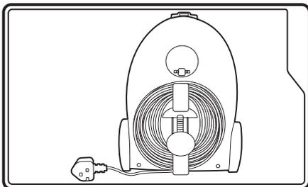
For quick release of the cable, rotate the lower portion back half a turn.
