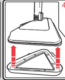
Fit the cloth to the floorhead using the grips on the underside of the floorhead. If cleaning carpets, the carpet glider (28) should be attached to the floorhead.
