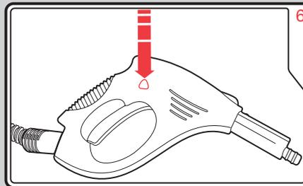
Press the steam trigger lock (12) to allow the steam trigger (15) to be operated. When not in use, press the lock 'on' to prevent accidental release of steam.
