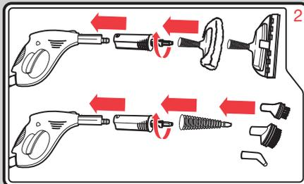
Push the upholstery nozzle (17) or jet nozzle (29) onto the accessory adaptor (21) and turn in a clockwise direction to lock into place.
