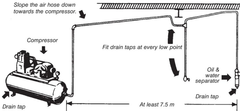
The oil and water separator should be at least 7.5 m from the compressor.
