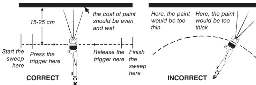
The distance from the nozzle to the work surface should be between 15 and 25 cm, depending on the type of paint and the air pressure. The coat of paint should be even and wet (shiny). Overlap the previous sweep to ensure an absolutely even finish.
