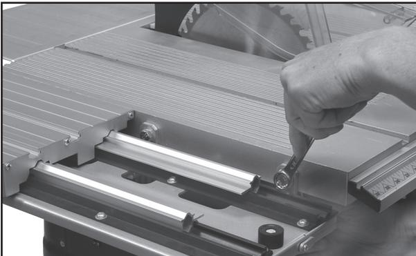
Replace the table saw's aluminium mitre guide slide with the longer aluminium slide which comes with the mitre guide.
