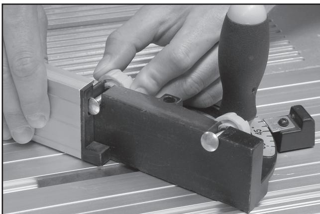
The mitre guide can be slid into one of the slots on the slide and locked by tightening the handles on the mitre guide.
