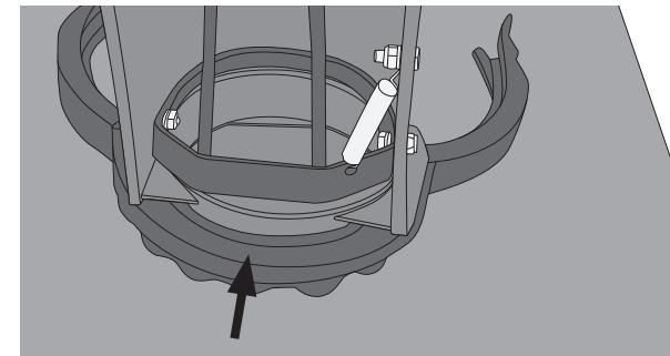
3. Place the chute over the coupling on the snow blower with the opening facing forwards.
