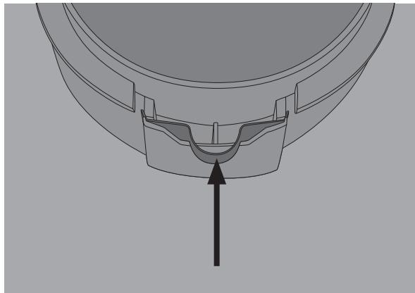
2. Lay out the locking collar as it is to be fitted, i.e. with the clamp on the right hand side.
