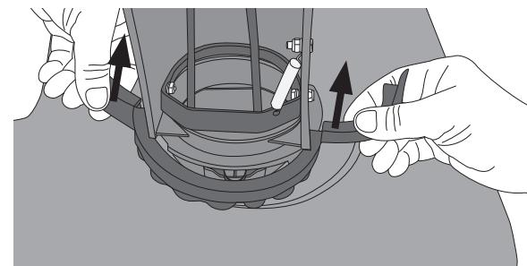
6. Lock the ends of the collar together using the snap lock. Turning the chute to the side will help you access the snap lock more easily.
