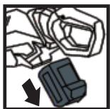
Remove battery before adjusting or cleaning, and before leaving the machine unattended for any period.
