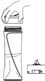
3. Turn the beaker upside down and screw the blade attachment onto the motor unit.
