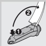
**1** Press the release button and open the cover of the cartridge compartment.
