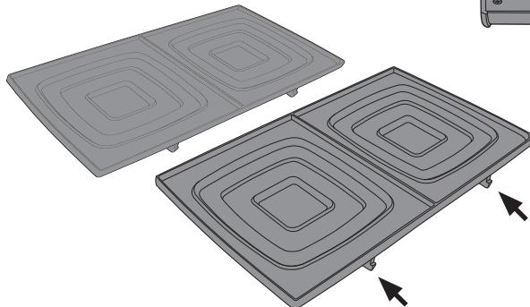
4. Position the front lock lugs over the latches at the front of the sandwich toaster, and then carefully press the plate until it is properly fitted.
