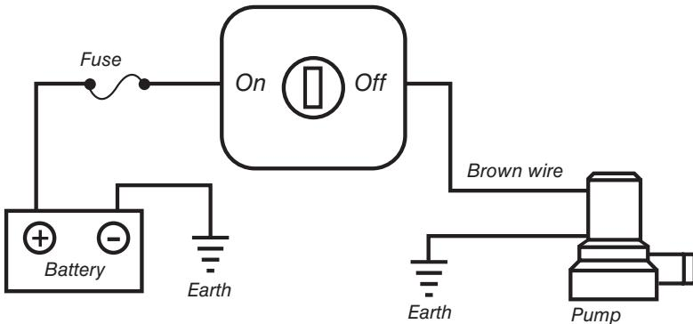
The pump must be switched on and off manually, using the on/off switch.
