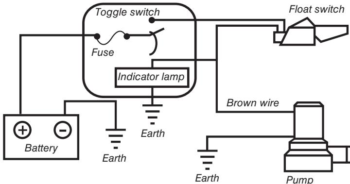
The pump is turned on or off automatically as the water level in the bilge rises or falls. The pump can also be activated by using the toggle switch on the control panel.
