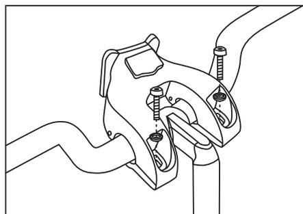
**Step 3.** Position the webbing strap so that the bolts pass through the strap holes and clamp holes and screw on the nuts. Make sure that the bracket is tight before hanging the bag on it.
