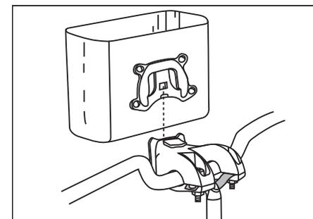
**Step 5.** To remove the bag, press and hold in the release button on top of the bracket and lift the bag up.
