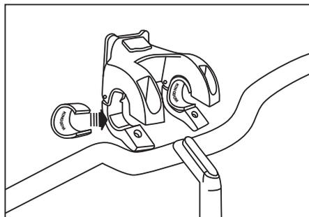
**Step 2.** Insert the bolts through the washers and holes on top of the clamps.
