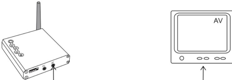
4. Connect one end of the power adaptor to the receiver and the other end to the wall socket.
