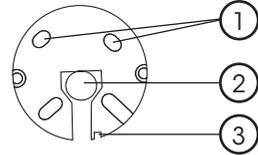
5. Pull the power supply cable through the centre hole (2) and screw the plastic backpiece onto the wall. Make sure that the drainage hole (3) in the plastic backpiece is at the bottom.
