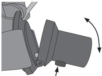
3. Push the holder back into the torch and look at the arrow on the holder to make sure that it is pushed in the right way.
