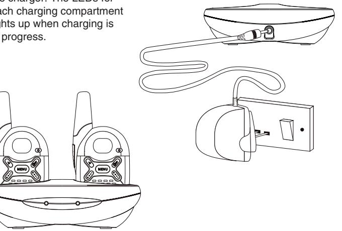
**NOTE!** Use only the included battery pack in the device when charging on table stand. Charging of other batteries does not work.
