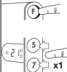
Hold down on “F” and press once on “7” or “5” to override the current active period, or the next period of temp. reduction. The lamp is lit steadily for the period in question. Temp. reduction will resume as usual from the following period.
