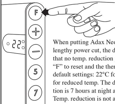
When putting Adax Neo into operation or after a lengthy power cut, the display will flash, showing that no temp. reduction programme is active. Press “F” to reset and the thermostat will revert to the default settings: 22°C for normal temp. and 15°C for reduced temp. The duration of temp. reduction is 7 hours at night and 5 hours during the day. Temp. reduction is not activated.
