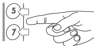
Hold down on “7” or “5” until the green lamp is extinguished.
