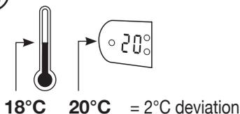
Should the actual room temperature and the Neo's setting not correspond, Neo should be calibrated. First let the heater work steadily at the same temperature setting, preferably for at least 24 hours, keeping doors and windows closed. This makes certain that it is Neo that is controlling room temperature. Sudden, big changes in outdoor temperature may affect calibration, making it less precise.
