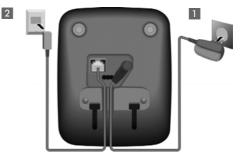
Only use the mains adapter and phone cord supplied. Pin connections on telephone cables can vary (pin connections → page 44).
