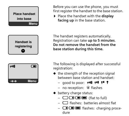
If you have purchased a **model with multiple handsets**, repeat the registration process for each handset. Handsets are assigned the lowest available internal number (1-4). If more than one handset is registered to the base station the internal handset number appears on the display, e.g. INT 2. If the internal numbers 1–4 are already assigned to other devices, the number 4 will be overwritten.
