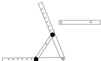
Use the long struts for roof mounting at angles of 30–70°.
