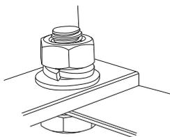
1. Fasten the panel mount onto the frame of the solar panel using the provided nuts, bolts and washers.
