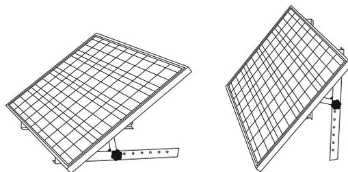
2. Mount the solar panel on a roof or wall and tilt it to a suitable angle by inserting the provided struts into the appropriate holes in the mount.
