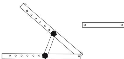
Use the short struts (230 mm) for wall mounting at angles of 15–40°.
