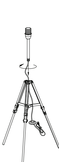
2. Screw the lamp holder tube onto the tripod.
