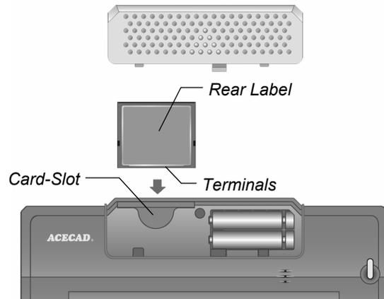
Note! The optional memory card must be Type I CompactFlash (CF) memory card.
