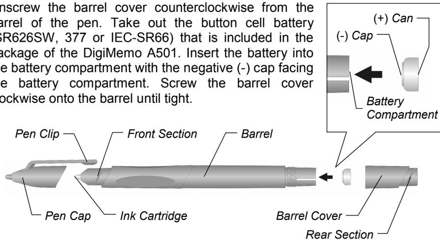
Note! Incorrect battery installation will result in the malfunction of the digital inking pen.
