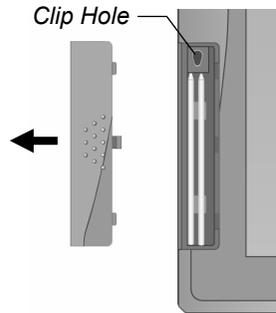
To replace the ink cartridge of the pen, you may use a small clip to gently pull the old one out. Then insert a new one and press the cartridge tip firmly against a hard surface until it snaps into place.
