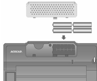
Note! Incorrect battery installation may damage the digital pad.
