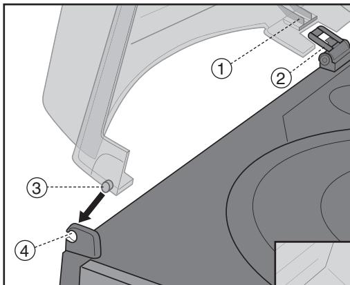
2. Fit the cover (1) on the hinge fitting (2) but not all the way down.
