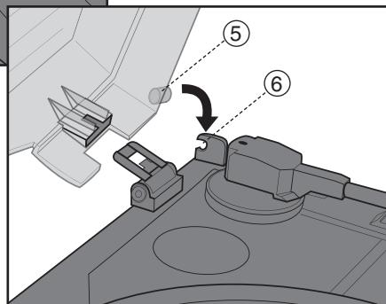
3. First set the cover's left pin (3) in the record player's left fixing (4) and then push the cover's right pin (5) carefully in the record player's right fixing (6).
