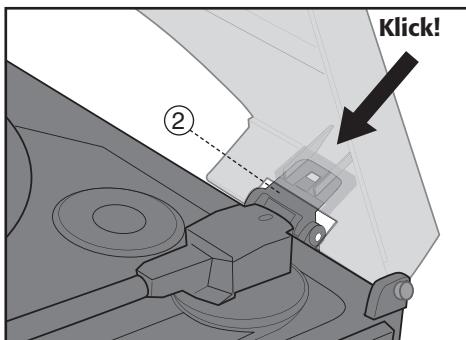
4. At the same time press down the cover on the hinge fitting (2) until it is locked and a click sound is heard.
