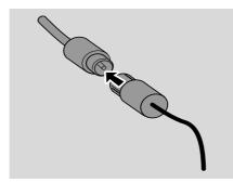
**Note:** If you are using a cable antenna system or an outdoor antenna, fit the antenna plug, instead of the wire antenna, to FM ANTENNA.
