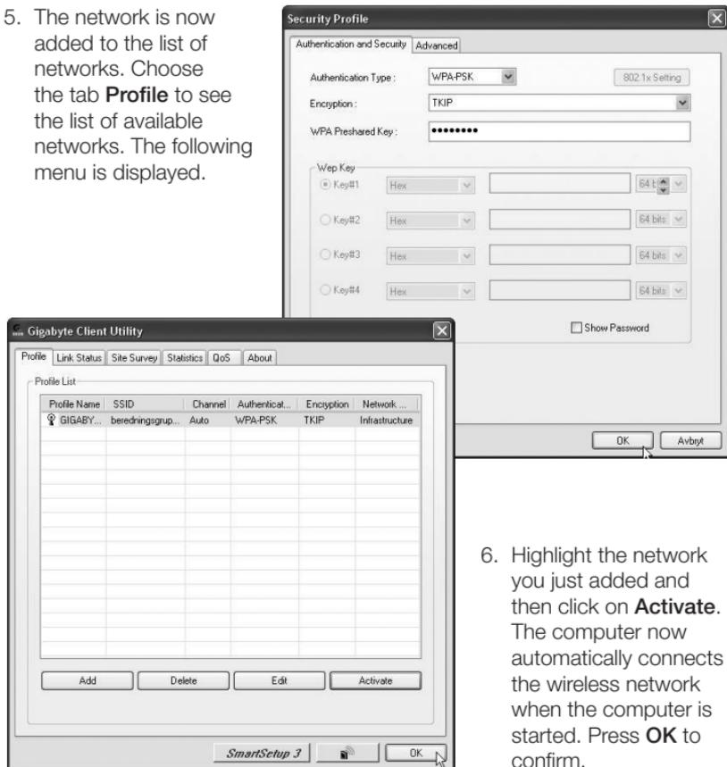
6. Highlight the network you just added and then click on **Activate**. The computer now automatically connects the wireless network when the computer is started. Press **OK** to confirm.
