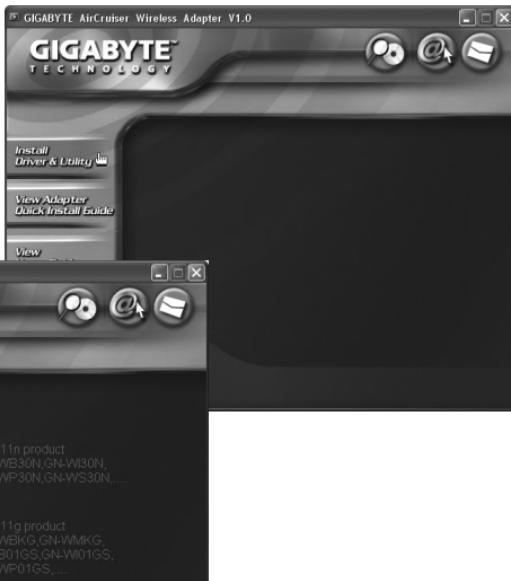
2. Click on **Install Driver & Utility** and then the button **N300 series** to install the configuration program.
