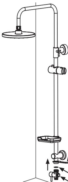
13. Refit the diverter to the bottom of the slide rail using a washer.
