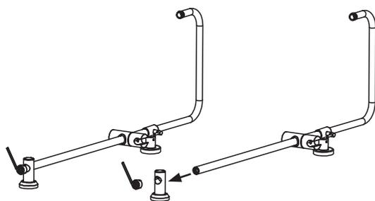
2. Using the included hex key, undo the screw and remove the bushing in the bottom of the slide rail. It will be easier if you ask someone to hold the rail for you while you undo the screw. Remove the bushing and swivel nut.
