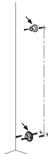
6. Drill mounting holes in the wall as shown above.
