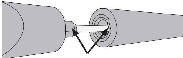
2. Slide the thermometer back into the spatula, it only fits one way, the bevelled edge of the thermometer fits against the corresponding edge in the spatula.
