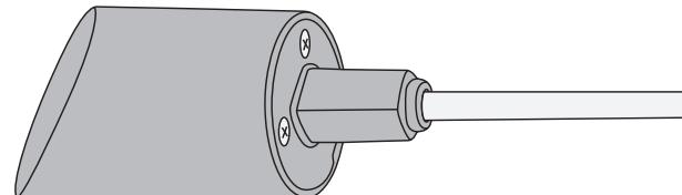
1. Remove the two screws holding the battery cover in place.
