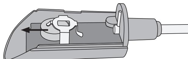
3. Carefully slide the battery out using an appropriate implement.
