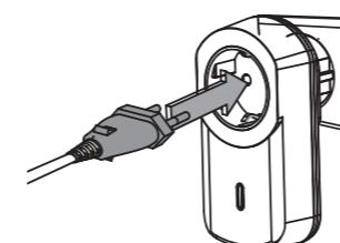
6. Connect a light to the receiver and check that the light is switched on.
