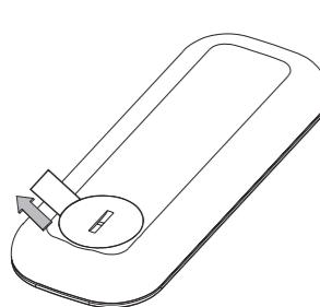
1. Remove the plastic tab from the back of the remote control to activate the battery.
