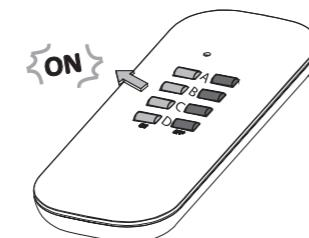
5. Single-press one of the on-buttons on the remote control (A, B, C or D). The LED on the receiver will shine steadily once the remote control has been paired.
