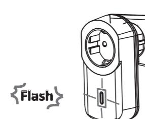
4. The LED button will start flashing slowly. The receiver is now in learning mode and ready to be paired with the remote control.
