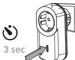
3. Hold in the button on the front of the receiver for at least 3 seconds and then release it.
