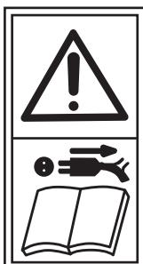
Always switch off and remove the plug from the mains before cleaning or maintenance.
