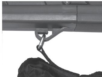
5. Hook the shoulder strap onto the motor housing. Adjust the length of the strap to suit the operator.
