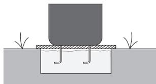
5. Use a spirit level to try and stand the letter box as vertical as possible. Fine-adjustments can be made later using the nuts on the ground anchor bolts.
