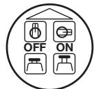
Never switch off the compressor by pulling out the plug or using the isolator switch (if fitted). Always use the ON/OFF button on the compressor.
