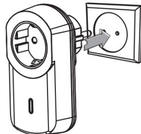
2. Plug the receiver into a wall socket.
