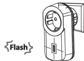
4. The LED button will start flashing slowly. The receiver is now in learning mode and ready to be paired with the remote control.
