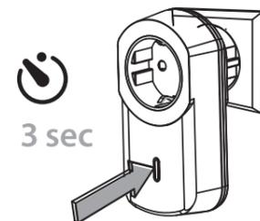
2. The LED in the button will start flashing slowly. The receiver is now ready to delete the remote control.
