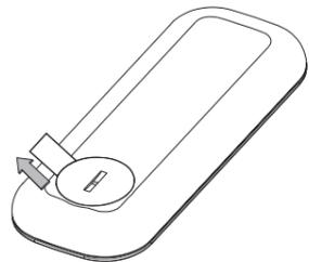
1. Remove the plastic tab from the back of the remote control to activate the battery.
