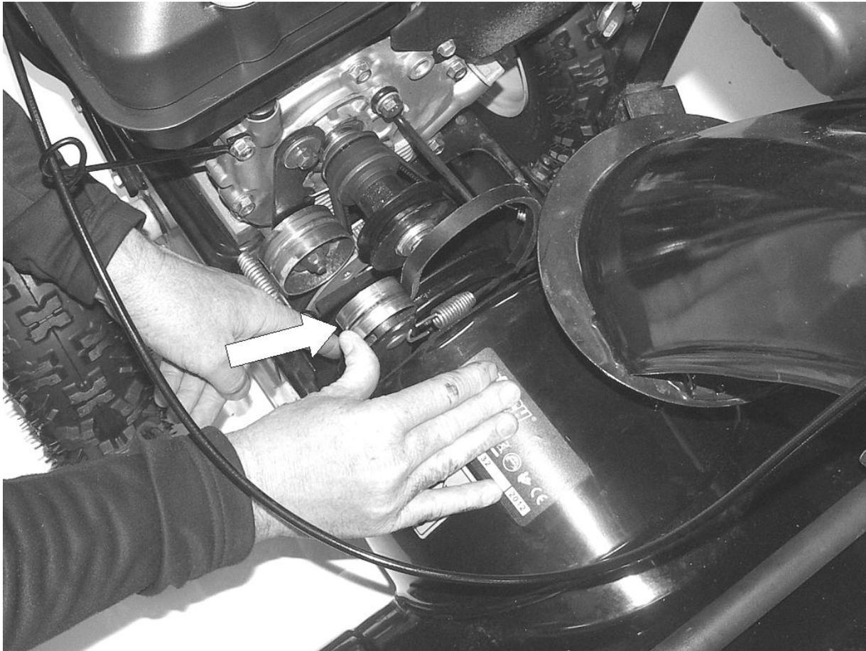
9. Pass the drive belt over the lower pulley once the guide wheel/brake has been moved. Note: This view is from below the snow blower.
