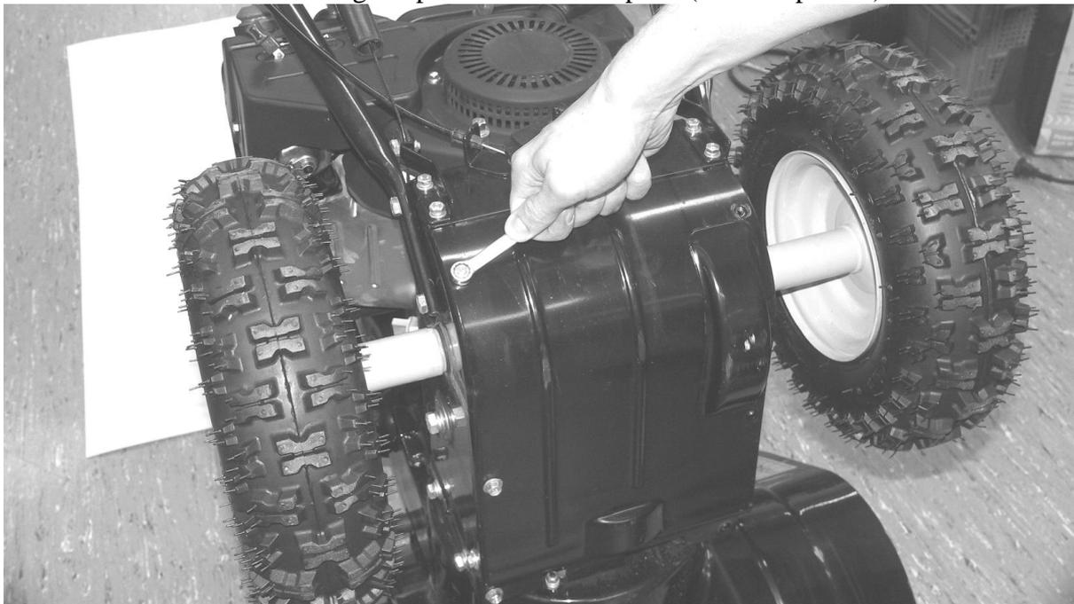
4. Slacken the auger drive clutch wire connected to the left handle. Remove the s-hook from the connector plate.
