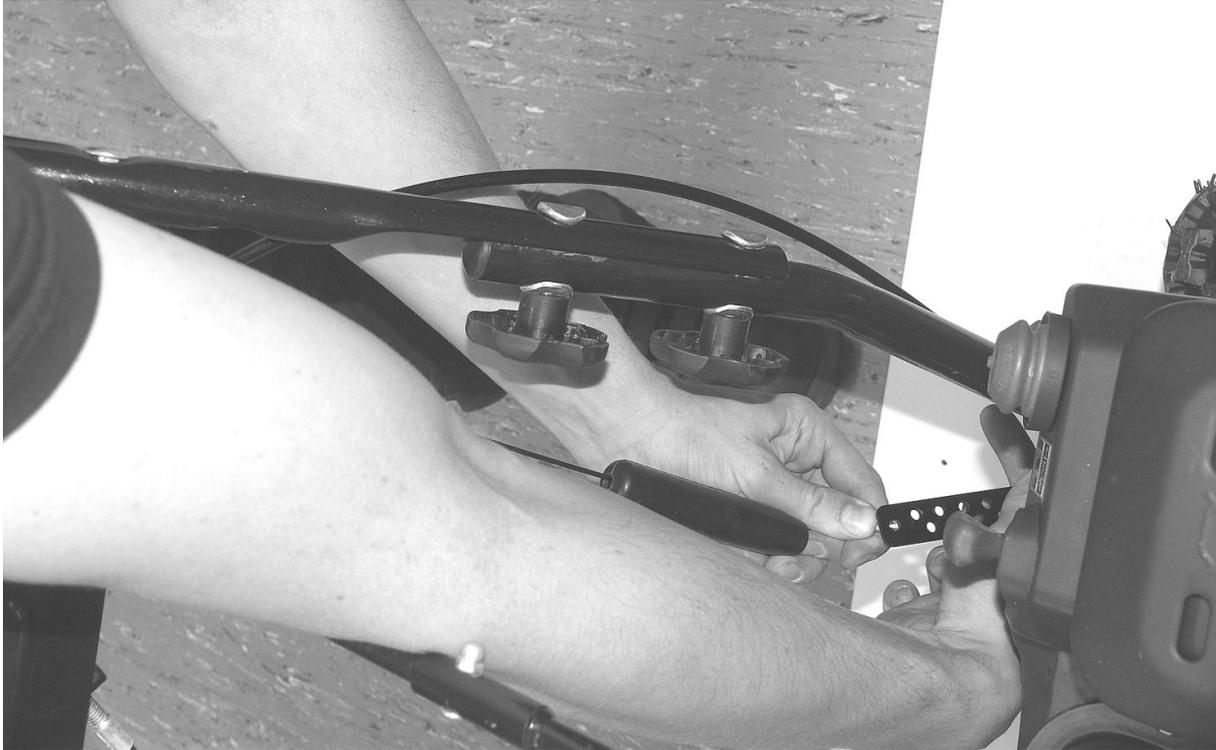
5. To access the drive belt the snow blower needs to be opened up in the middle. Return the snow blower to its normal upright position and remove the uppermost of the two bolts just behind the impeller housing on both sides. The two lower bolts do not need to be removed, just loosened (13 mm spanner).
