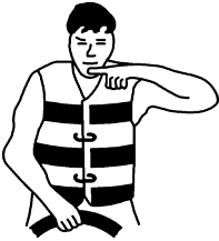
Cut engine: point to chin using forefinger
