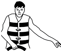
Return to launch: circular motion with forefinger pointing down
