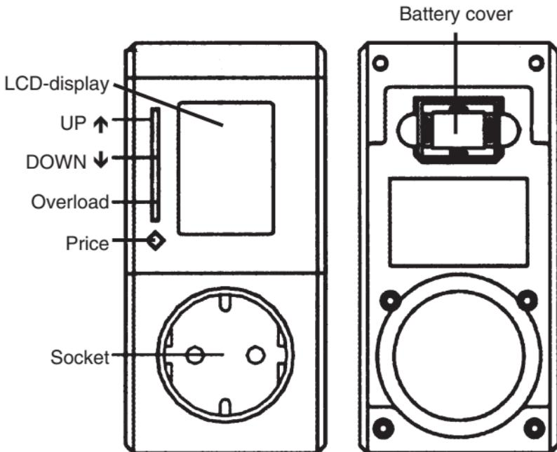
PM - 300 measures how much energy an electric device uses. The electricity meter can calculate the total cost of running a device by entering the price per kWh. It can also register possible overload. To be able to use this electricity meter in the best possible way we recommend that you read the entire manual before use.
