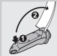
**2** Press the release button and open the cover of the cartridge compartment.
