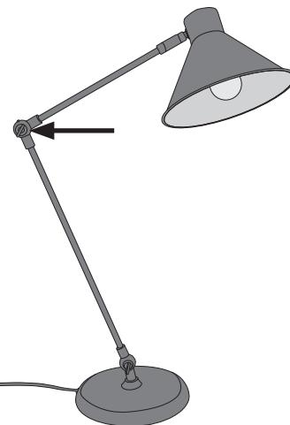
The screw in the joint of the arm needs to be undone before the arm can be adjusted. Remember to tighten the screw again afterwards.
