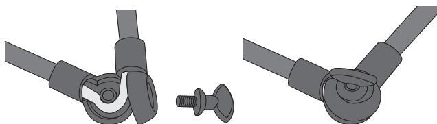
The sections of the arm need to be screwed together. Make sure that the power cable is not crushed.
