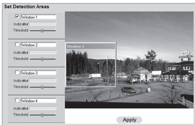
**Note: Motion detection can besides moving objects also react on rapid changes in light. It is therefore recommended that the function is only used on cameras indoors.**
