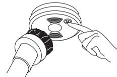
**WARNING:** Do not test the alarm using naked flames, these can damage the alarm and are dangerous. We do not recommend that you test the alarm using smoke as results can be misleading if the correct test equipment is not used. The test button tests all the necessary functions of the smoke alarm.
