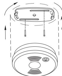
**Handy hint:** Before attaching the mounting plate to the ceiling, you should make sure that the radio signal is within the range of any other interconnected alarms. Try changing the position of one or several of the alarms if they are out of range (refer to *Test and maintenance*).
