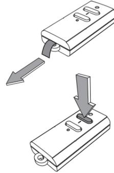
3. Press the on-button on the remote control to link it to the receiver.
