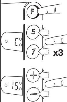
Hold down on "F" and press 3 times on "7" eller "5" depending on which you wish to change. When "°C" flashes in the display, release "F".
