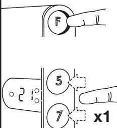
Hold down on "F" and press once on "5" or "7" to override the current active period, or the next period of temp. reduction. The lamp is lit steadily for the period in question. Temp. reduction will resume as usual from the following period.
