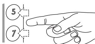
Hold down on "7" or "5" until the green lamp is extinguished.
