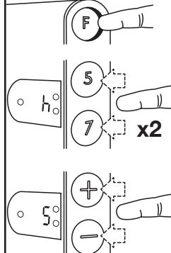
Hold down on "F" and press twice on "7" or "5" depending on which you wish to alter. When "h" (hour) flashes in the display, release "F".
