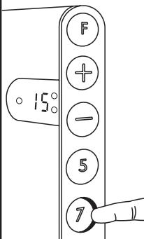
At the time you wish temp. reduction to start, press "7" until 15°C is displayed. The green lamp (B) will now flash slowly to indicate that temp. reduction is active. The temperature is lowered to 15°C for the next 7 hours. This will now be repeated at the same time every night.
