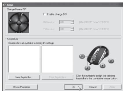
Open “X7-jump” (properties) by right-clicking on the mouse icon and choose X7-jump, click on the desired button (2 – 5) and click on the functions key (on the keyboard) that you wish to correspond to the desired mouse button.
