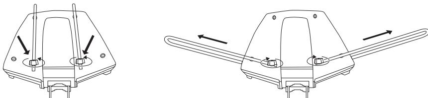
1. Loosen the four wing nuts (two on the top and two on the bottom of the aerial).
