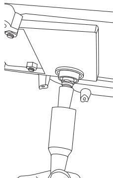
2. Connect the other end of the coaxial cable and the 12 V power cable to the splitter filter.
