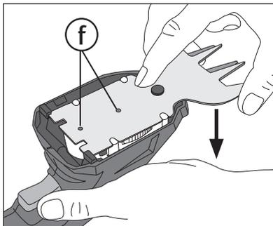
5. Then fit the shoe back onto the trimmer by sliding it in the direction of the arrow as shown in the picture.
